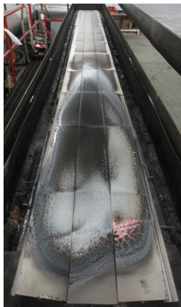
Photo No. 4 Exposed Surface of the Test Specimen (Post-test)
